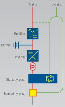
Double-Conversion On-line Technology with isolating transformer
