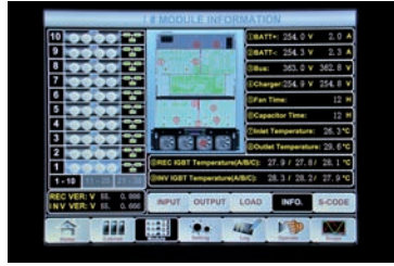
Total control and access of all modules parameters. Total management of all internal temperature for high performance control of fan speed and for smart parallel function management.
